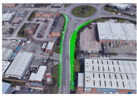
Complementary to the link road, widening the entry and exit on the A633 southern arm of Taylors Lane roundabout, extending the 2-lane sections by 150m in both directions.
